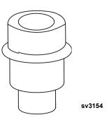
1. Remove check valve and tube assembly.
